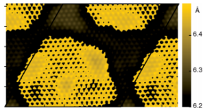
Fig. 2 Simulated STM using Tersoff–Hamann approximation at a bias of +1.0 V. Color bar is in units of Å relative to the topmost Cu layer, the x and y axis ticks at intervals of 10 Å. Black lines indicate the unit cell.
